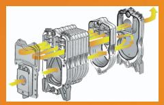
A 3-pass design is the most efficient way to get the maximum amount of heat from the fuel. It contains three times as much interior heating surface compared to a single-pass boiler.
