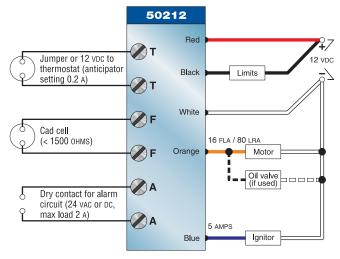
**Warning** — Do not ground power common leads to chassis. Route Red wire and limit circuit wire separately all the way to the DC power supply positive terminal. Route White wire and common from motor/ignitor/valve separately all the way to the DC power supply negative terminal. You must do so to ensure reliable control operation. DO NOT jumper these wires in the burner junction box. Size all wiring per applicable code requirements.
