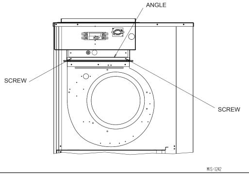
Power supply wiring can now be made to the heat package. Route the low voltage three pin plug through the wire restraints and plug into mating plug in back of control panel. (See Figure 6.) This connection supplies the low voltage control circuit to the heat package from the heat pump control circuit.
