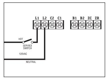
STEP 1 Connect 120 VAC Hot to terminal L1. Connect 120 VAC Neutral to terminal L2. Disconnect means and overload protection as required (provided by others).
