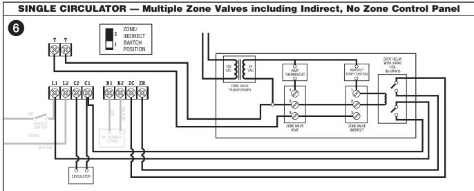
NOTE: When using zone valves for both heat and indirect, the calls must be separated in order to prioritize indirect calls. This can be accomplished by using a general purpose relay as shown above. However, for ease of installation, a zone control panel is recommended (see wiring diagram 7 on next page).
