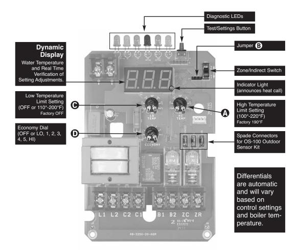
**NOTE:** Settings can be checked using the TEST/SETTINGS Button. See page 11 for details.
