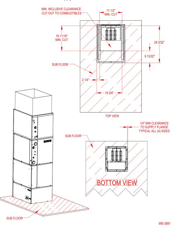
FIGURE 3 Supply Duct Floor Penetration
