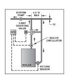
**Recommendation 3** is used when the return water temperature goes below 135°F for prolonged periods of time. This is also primary-secondary piping, but includes the addition of a 3-way valve, return water sensor and boiler-mounted RTC Return Temperature Control.
