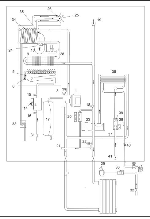
**Note:** Pressure Relief Valve (#22) should be piped to a drain or to the floor as close as possible to a drain.
