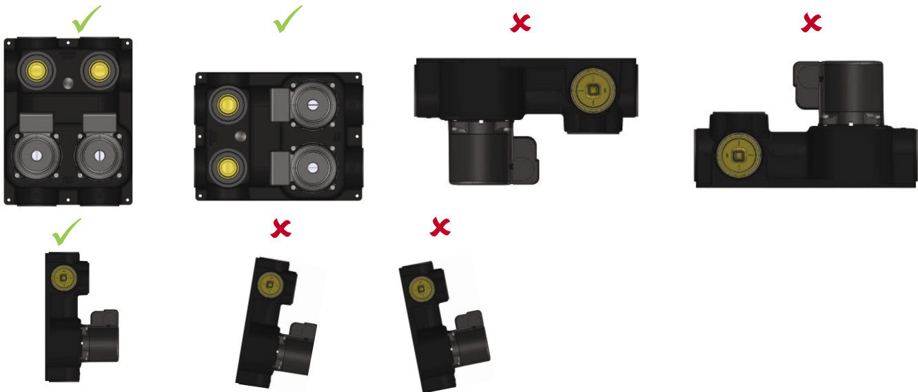
Figure 4: Acceptable mounting positions for Flo-Link and GPM series flow centers
