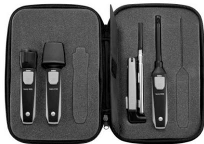
**Testo 405 I - Hot-wire Anemometer Smart and Wireless Probe**
