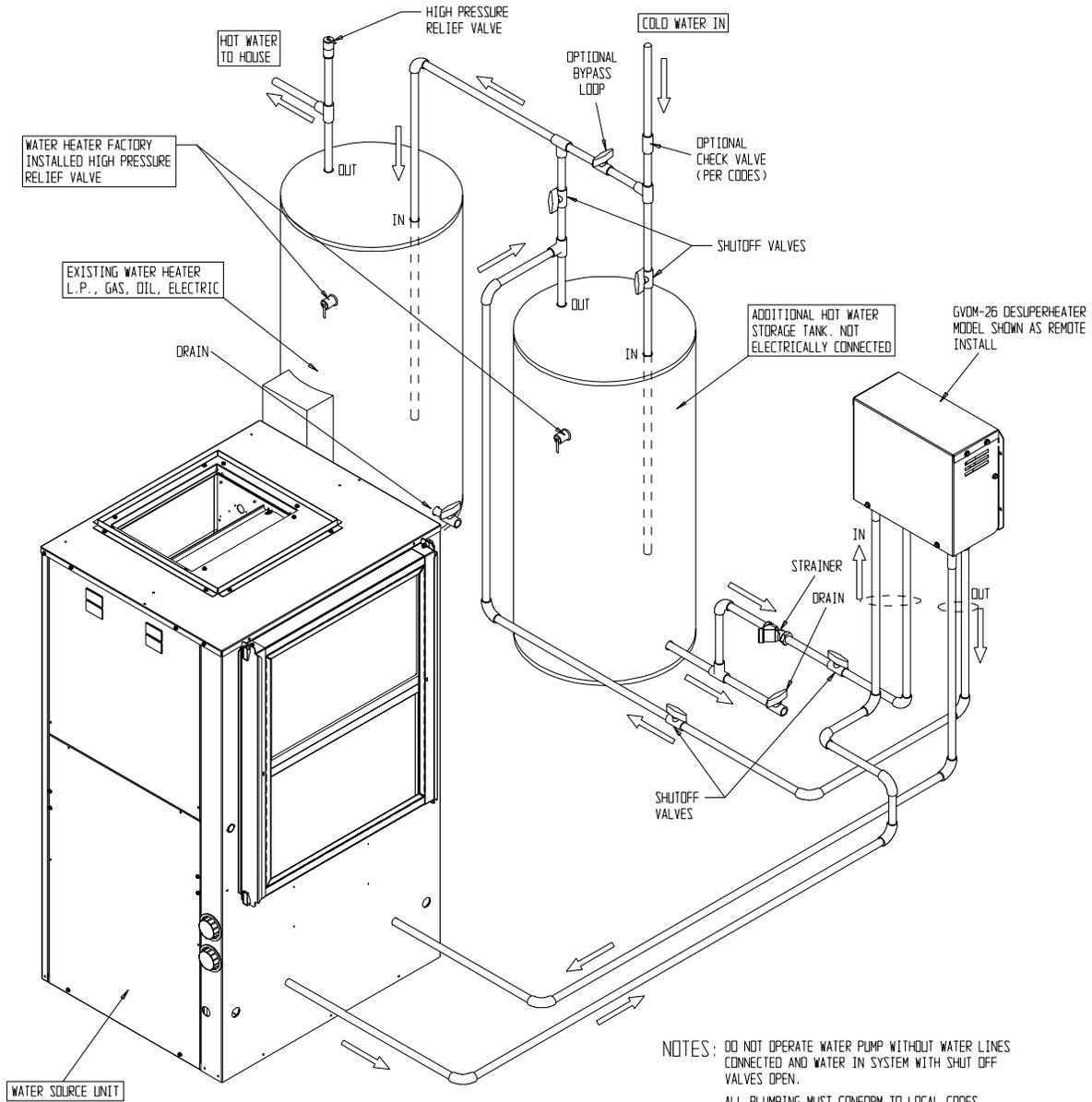
NOTES: DO NOT OPERATE WATER PUMP WITHOUT WATER LINES CONNECTED AND WATER IN SYSTEM WITH SHUT OFF VALVES OPEN.
