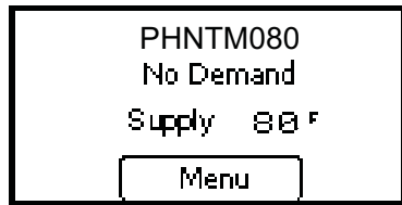
FIGURE 11.2a: HOME SCREEN AT POWER-UP (No Call for Heat)
